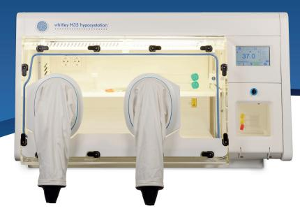
The Whitley Hypoxystation creates physiological cell culture conditions with regard to temperature, humidity and gas atmosphere. The uniquely low gas consumption  $(N_2 \text{ and } CO_2)$  of a Hypoxystation is significant because:
